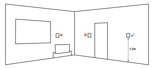
The performance of room thermostats is affected by airflow in the room. If a room thermostat is positioned incorrectly, then the airflow across it will not be representative of the airflow in the room in general and, therefore, the
